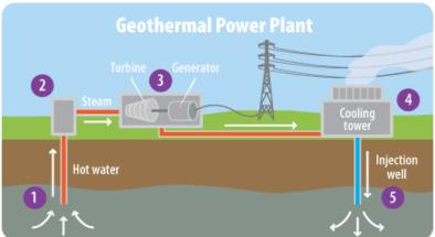
Figure 33. Geothermal Power Plant.
